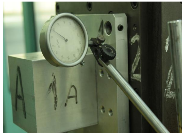
Fig. 3 Measuring deviations on machine Z axes for the detachable pallet „A” in device „2” in repeatability case
