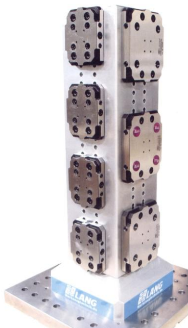
Fig. 1 Modular fixture device fixed on the pallet, on which are positioned the detachable plates[10]
