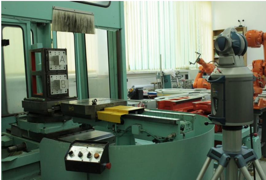
Fig. 4 Measuring of the modular fixture with Laser Tracker [5]
